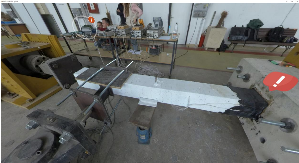
Figure 5.11: Column scene of the VT from the quasi-static test at IZIIS (after being repaired)
