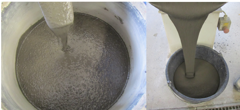
Figure 4.4. UHPC containing RHA after mixing in a Pemat ZK30 mixer.
