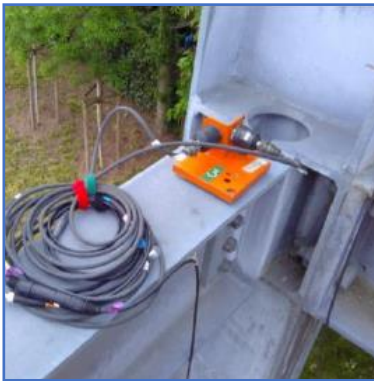
Installation with aid of magnets
